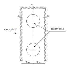
Figure 6 : The sub-soil reinforced by Jet Grouting at the cross-section at the Opera House (URMB 2010)
