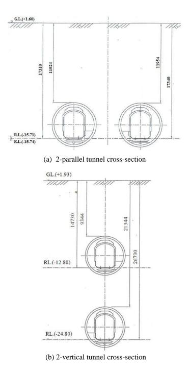
Figure 3 : Two typical tunnel cross-sections applied in the metro line No. 1 (URMB 2010)
