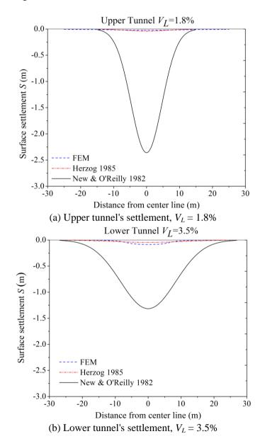
Figure 5: Surface settlement analysis for the study cross-section
